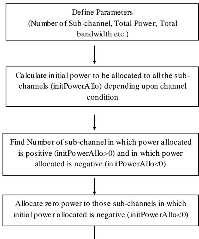
Thus capacity of channel is improved. Here we are giving flow chart for the proposed Water Filling Algorithm (WFA).
