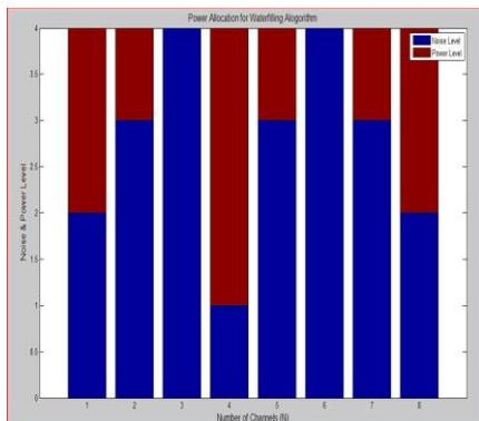
Figure 7: WFA for fixed noise power channels
