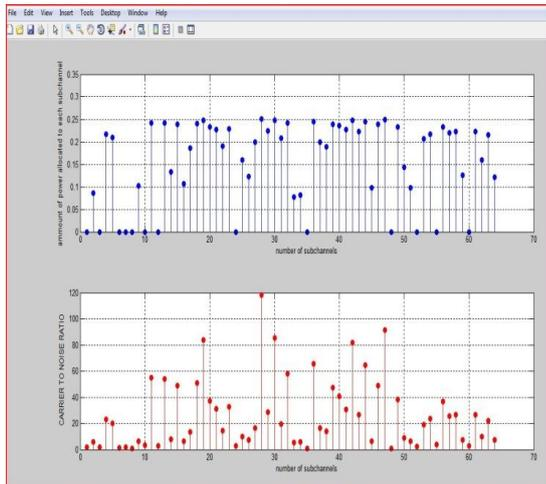
**Figure 7: Power Allocation for 64 sub-channels**
