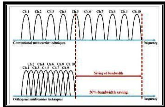
**Figure 2: FDM Vs OFDM**
