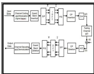
Figure 3: OFDM Communication System
