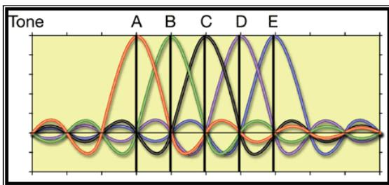
**Figure 1: OFDM Signal showing orthogonal Carriers**
