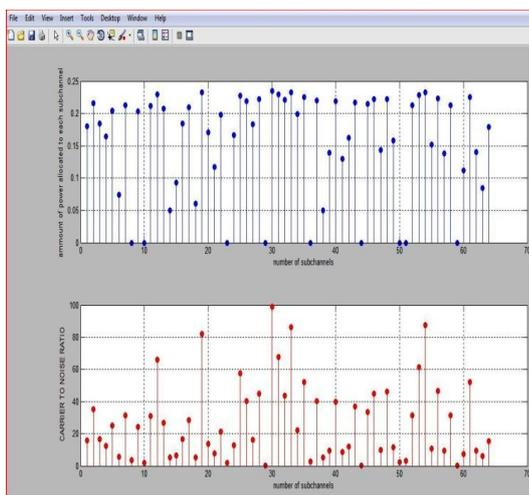
**Figure 8: Power Allocation for 64 sub-channels**
