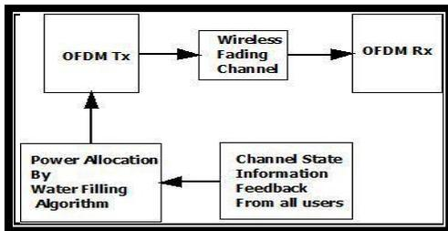
Figure 6: Working Operation of WFA
