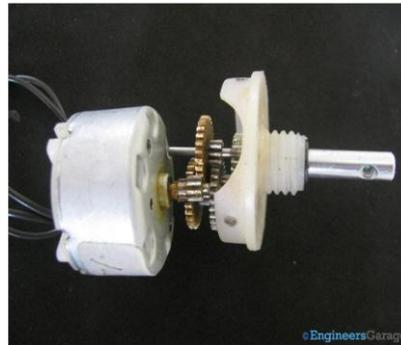
Fig.5 Gear mechanism to dc motor
