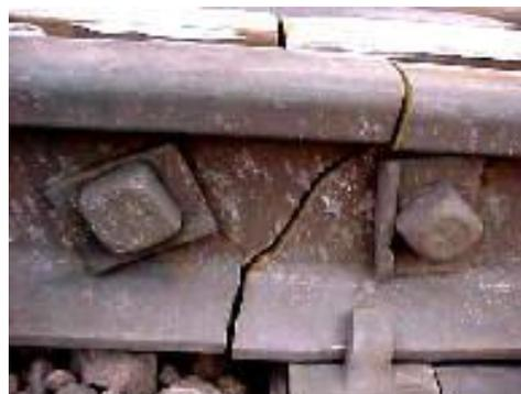
Fig.1 Cracks in Railway tracks
