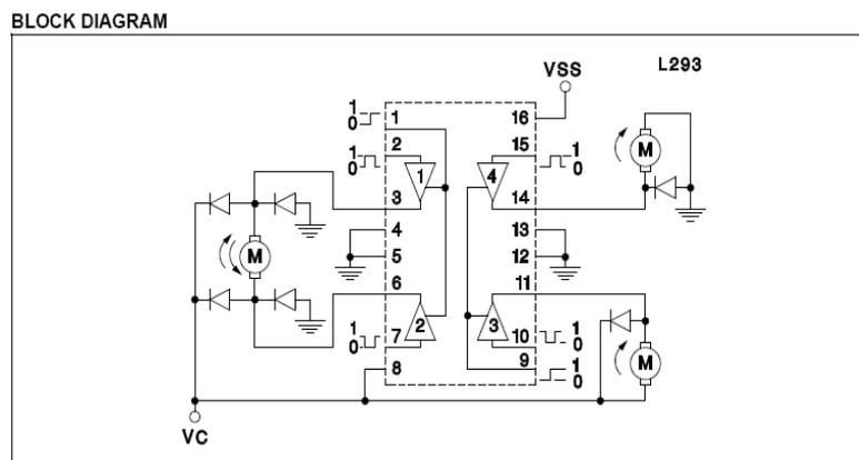
Fig.6 Block diagram of load driver L293
