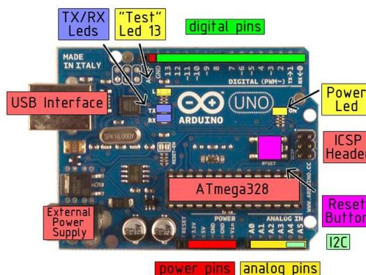
Fig.3 Basic Arduino UNO board
