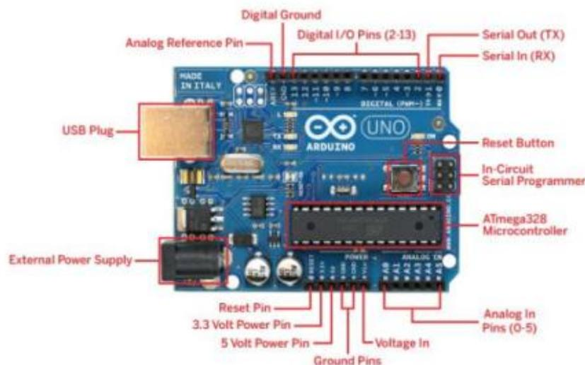
The Arduino Uno consists of 14 digital input/output pins (of which 6 can be used as PWM outputs), 6 analog inputs, a 16 MHz crystal oscillator, a USB connection, a power jack, an ICSP header, and a reset button.
